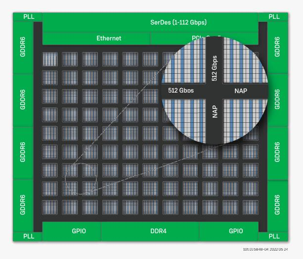
Figure 4 – 20 Tbps 2D NoC
