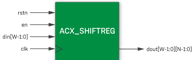
Figure 36: ACX_SHIFTREG Logic Symbol
