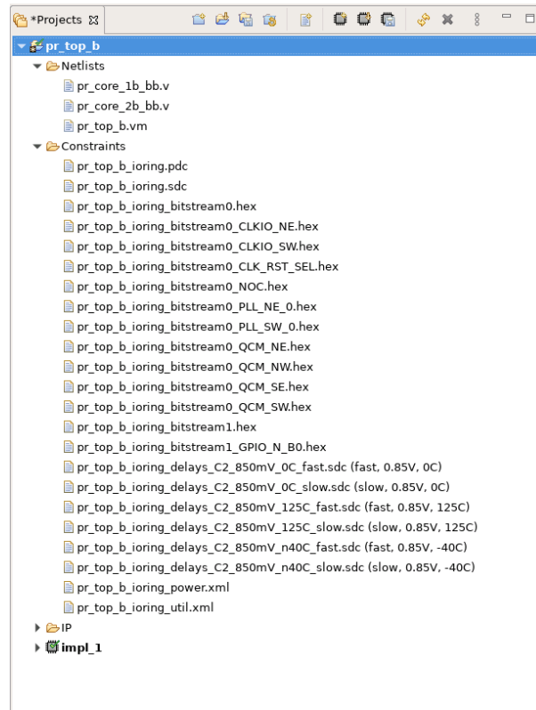
Figure 280 - PR Core Source Files Example
