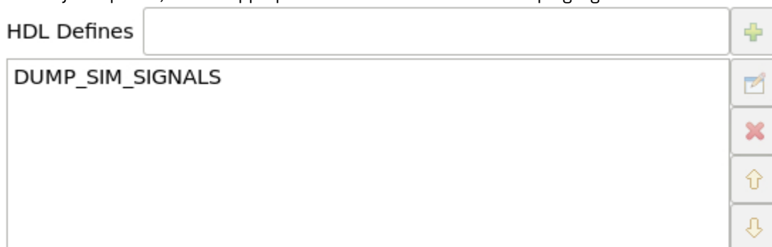
Figure 329 - Setting HDL Define to Dump Signals
