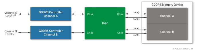
Figure 6 • Dual-Controller x16 Mode Block Diagram
