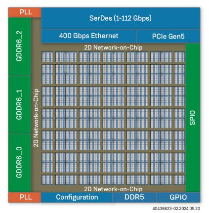
Figure 2 • Speedster7t AC7t800 FPGA Architecture Overview Block Diagram
