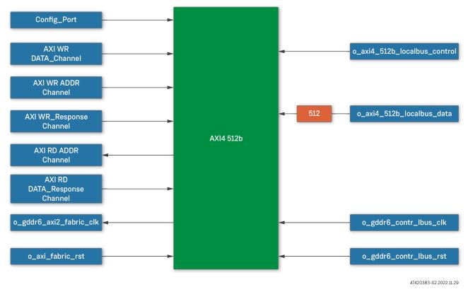
Figure 22 • AXI4-512b I/O Diagram
