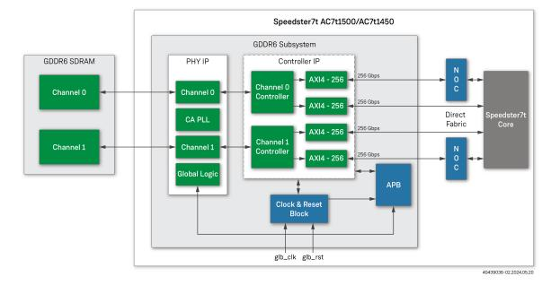
The following block diagrams show the GDDR6 subsystem in the Speedster7t AC7t1500, AC7t1450 and AC7t800 FPGAs:
